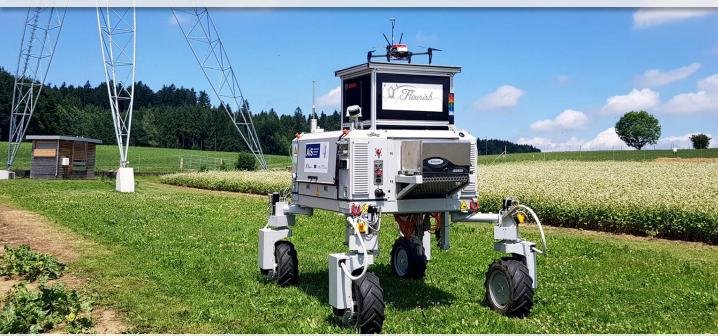
UGV acts as a **mobile docking** and **charging station** for UAV. During the missions, the UAV automatically lands and starts from the UGV to recharge its batteries. UAV can upload data on the UGV data analysis module
